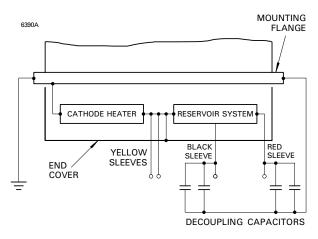
Fig. 2 CX1836X base connections
