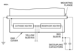
Fig. 1 CX1836 base connections
