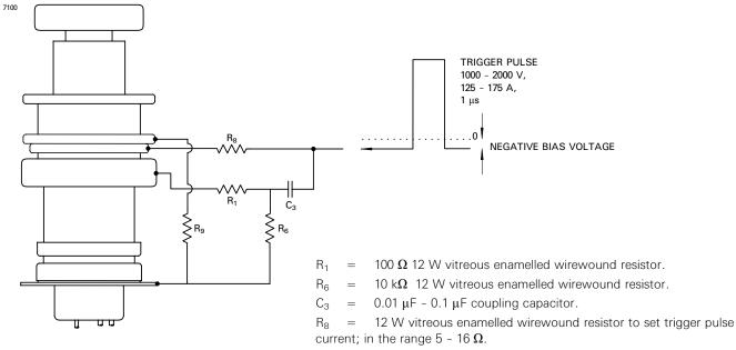
$R_9 = 1 \Omega$  to 10  $\Omega$  depending on degree of screening required; 12 W vitreous enamelled wirewound resistor or resistance wire (> 10 W).
